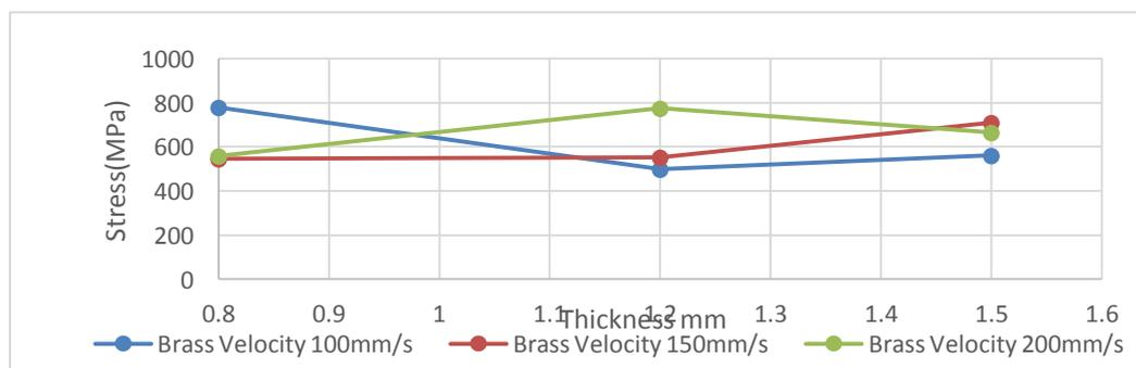
**Fig. 9 Effect of Blank Thickness on stress for brass material with change in different velocities**
