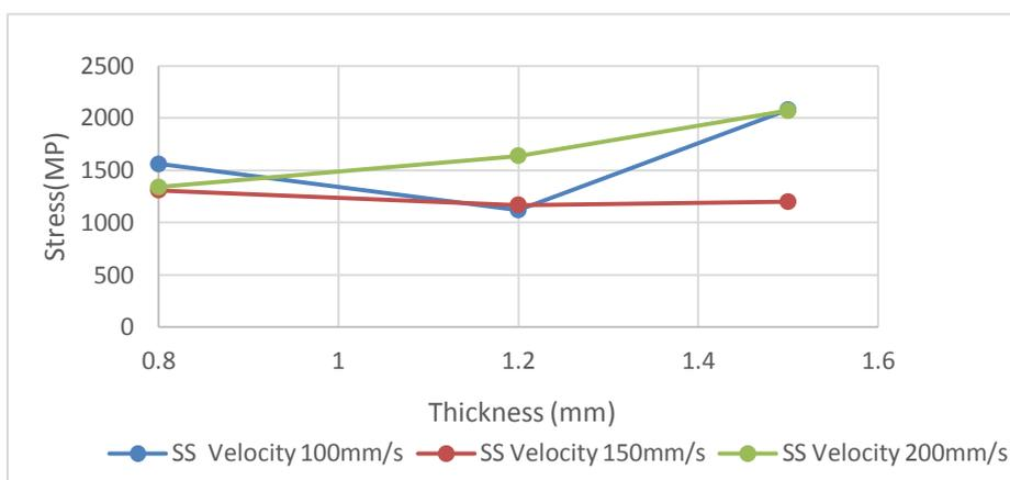
**Fig. 7 Effect of Blank Thickness on stress for Stainless Steel material with change in different velocities****3.3 SIMULATION RESULTS FOR BRASS BLANK MATERIAL:**
