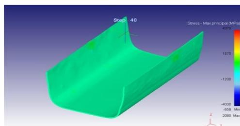
**Fig. 6 Stress variations in stainless steel of 1.5 mm thickness and 100 mm/s velocity**
