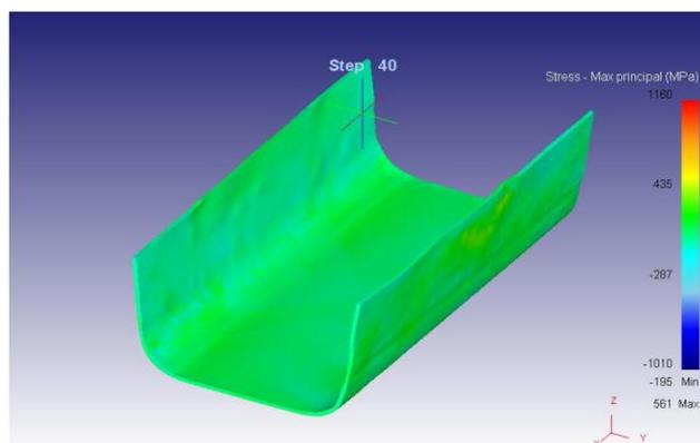
**Fig. 8 Stress variations in stainless steel of 1.5 mm thickness and 100 mm/s velocity**
