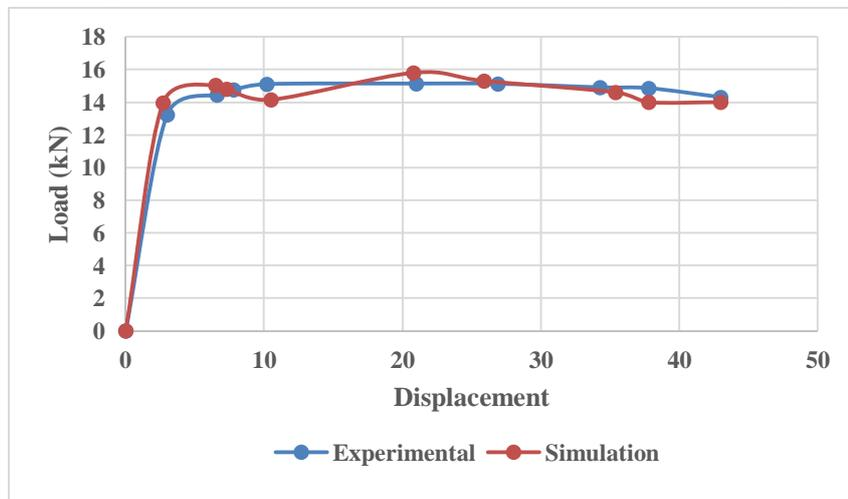
**Fig. 3 Variation of Load against Displacement for Stainless Steel with 1.5 mm thickness and 1.2 mm/sec Velocity**
