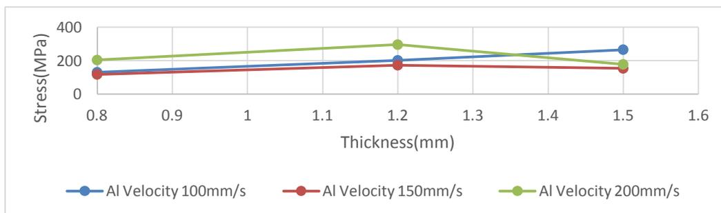
**Fig. 5 Effect of Blank Thickness on stress for aluminum material with change in different velocities**
