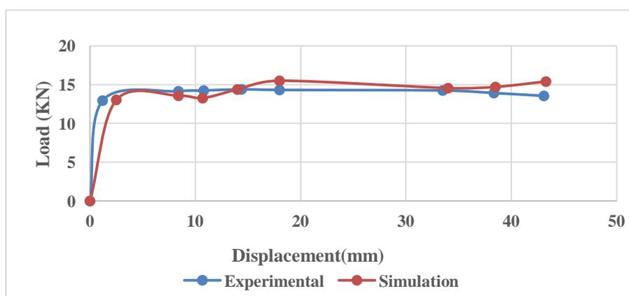
**Fig. 2 Variation of Load against Displacement for Stainless Steel with 1.2 mm thickness and 1.2mm/sec Velocity**
