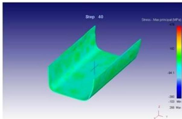
**Fig. 4 Stress variations in aluminum of 1.5 mm thickness and 100 mm/s velocity**
